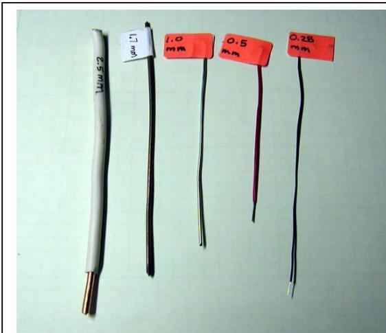
**Figure 1:** Set of five wire gauges
