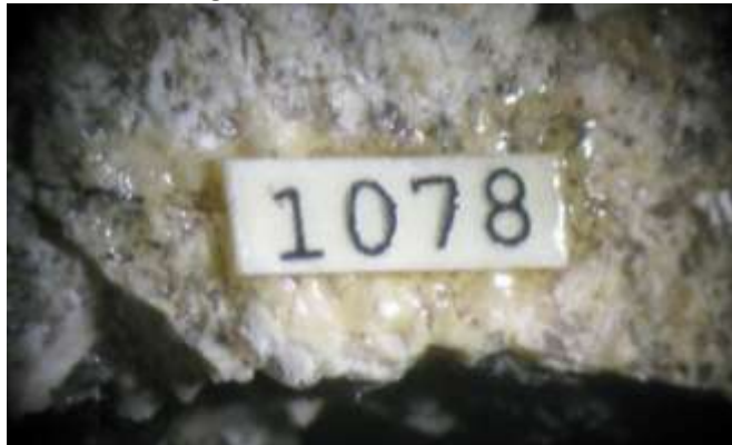
Specimen number attached with urethane conformal coating
